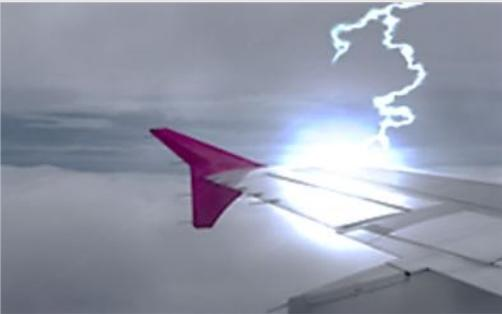
Each US aircraft is hit with lightning more than once a year. Aluminum allows the energy to travel along the skin and release back to the atmosphere. Composite structures cannot do this nearly as well and the potential exists for arcing close to fuel lines.
